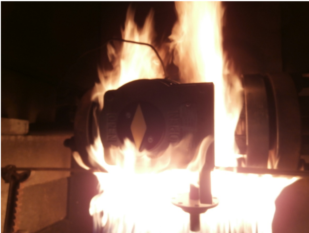
Test Valve During Burn
